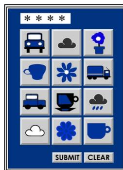
**Figure 2:** Password entry keypad, using pictures
